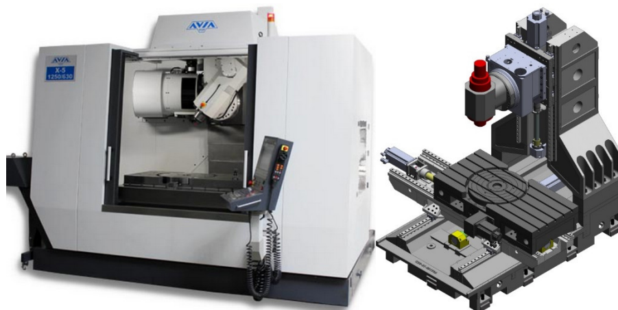
Figure 10. AVIA X-5 machining centre and its SolidWorks model.
